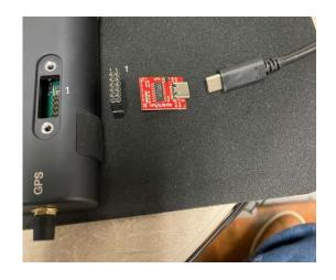
On the SparkFun module there is a voltage mode jumper labeled 5V and 3.3V. The default voltage setting is 3.3V. Leave this module in this default 3.3V position/mode.
