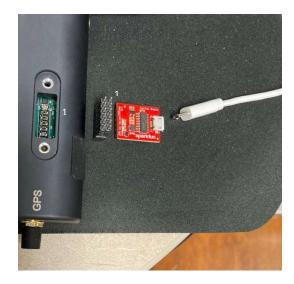
On the SparkFun module there is a voltage mode jumper labeled 5V and 3.3V. The default voltage setting is 3.3V. Leave this module in this default 3.3V position/mode.
