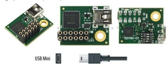
This module was the original module planned to be used for this purpose. It also provides a means to program and debug the Xilinx FPGA. This adapter/module is pin compatible with the connector on the Oxygen unit and plugs straight into place using the provided extension connector from Samtec, part# ESQ-106-44-L-D, as shown below:
